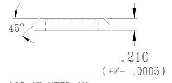
The Airo Tool Replacement Ring is used with the 3 piece Blow Pin Assembly. This assembly replaces the one piece pull up cutter. The illustration shows a 1.200 diameter. This is for an example the o.d.'s come in many sizes to fit your needs.
